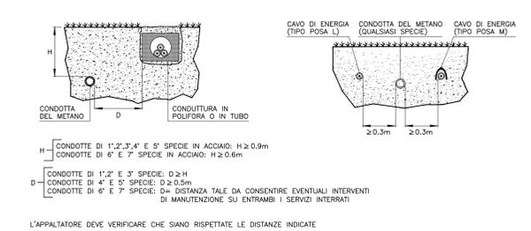
TIPICO POSA CAVIDOTTI INTERRATI BASSA TENSIONE
